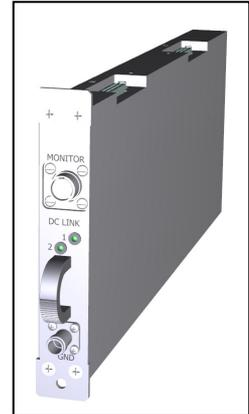
The TPS module is integrated in an IP67 small size aluminum container, made from solid, whose function is also to transfer the heat towards the cooling plate, on the front panel there are two status LEDs of the two power supply channels and a monitoring connector from which it is possible to check the internal power supply stages.
