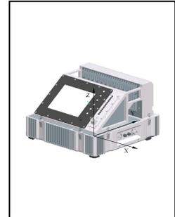
The AC/DC assembly is the main power supply provider of RFCT system, the converter topology is founded on a PWM, Current Mode Flyback that manages the required output power and provides isolation between the AC source and the Load. The mains input voltage is 100 to 242 Vrms, 47 to 63 Hz (without range switch), Pout up to 100W and Vout range from 24 to 28Vdc.
